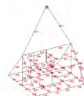
Figure 20: FE model - load case 2 - 3 temporary support points loading
