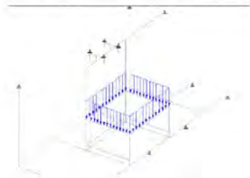
Figure 8.3: Strand model, manifold load
